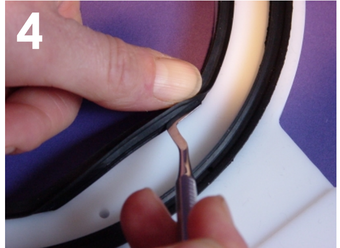
Insert the ring into the nut, use the flat end of the tool
